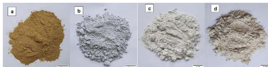
Dried raw appearances of: a) Dried and disaggregated clay; b) FGD residue; c) Soda-lime glass polishing waste; and d) OSR (Ornamental stone residue)
